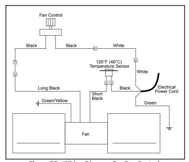
Figure 35. Wiring Diagram For Fan Control.
